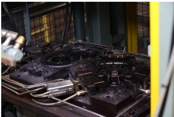
Metal mold for fabricating the rotor core
