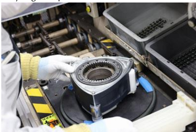
Gas seals are assembled by hand
