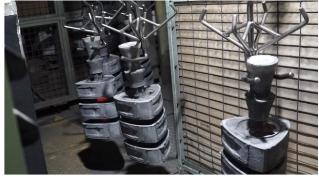
Rotor material taken out from a mold
