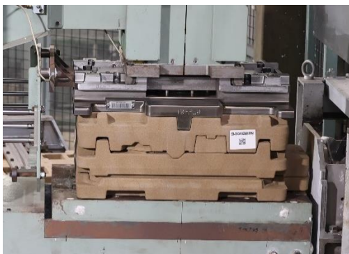
Upper gray component is a metal cooling plate
