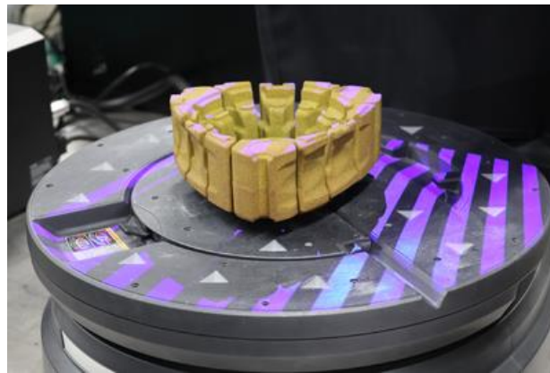
3D scan of a sand mold
